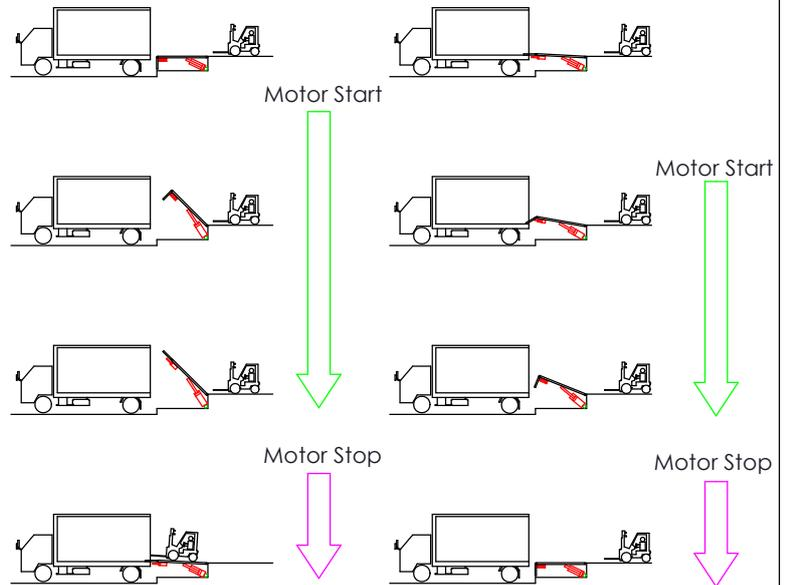
"Dock Leveller" Hydraulic Valves Diagram
